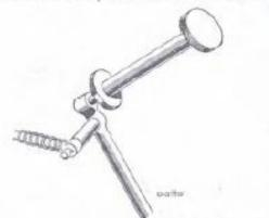
'The adjustable accelerator pedal on the Diatto chassis, giving two minimum settings
