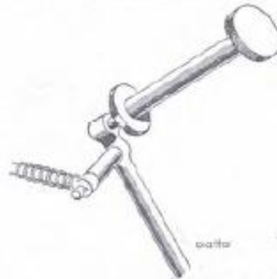
The adjustable accelerator pedal on the Diatto chassis, giving two minimum settings
