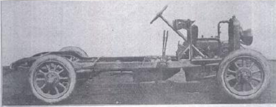
THE 25 H.P. DIATTO CHASSIS: Off-side view: The height of the radiator will be specially noticed.
